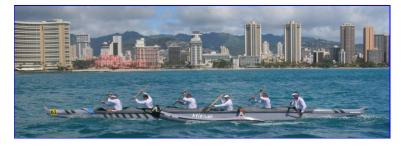
Outrigger Connection Mirage OC6 was designed to take advantage of the additional buoyancy of saltier waters. The increased hull width and more pronounced calabash in the centre of the canoe allows the canoe to accelerate faster, turn quicker, and pick-up waves a lot easier.
